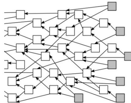
IOTA's Tangle and its typical tip sets (shaded). Each transaction approves two previous transactions. Once a transaction is sufficiently deep, it is considered confirmed.
